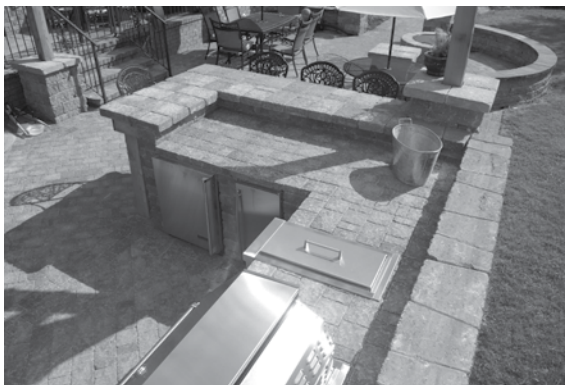
Figure 6-17: Appliances in an outdoor kitchen must be rated for outdoor use.
