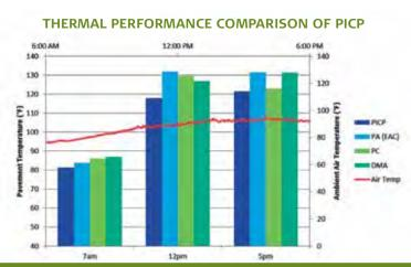
Figure 2. Thermal performance comparison of PICP, porous asphalt, pervious concrete and conventional asphalt with measurements taken on June 21, 2012.
