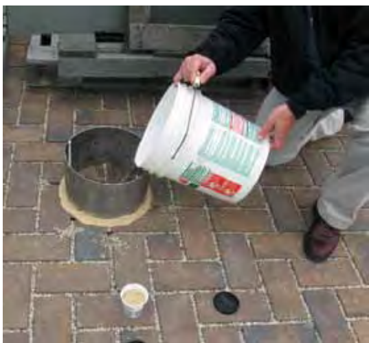
Figure 1. Test apparatus on PICP for measuring surface infiltration rate per ASTM C1701.
