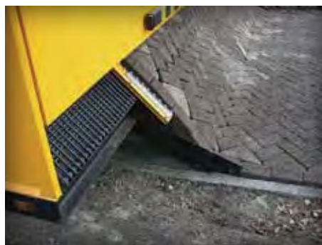
Figure 2. The machine follows curbs or guide string lines to locate the pavers against curbs. Five-sided "bishop hats" are used as edge pavers to close 45° herringbone patterns.
