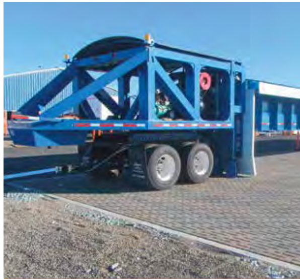
The Heavy Vehicular Simulator load tests permeable interlocking concrete pavement at UC Davis.
