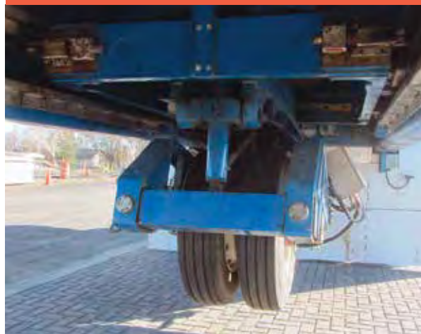
The Heavy Vehicular Simulator load tests permeable interlocking concrete pavement at UC Davis.
